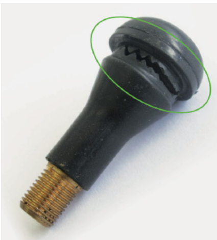
Old, torn valve
